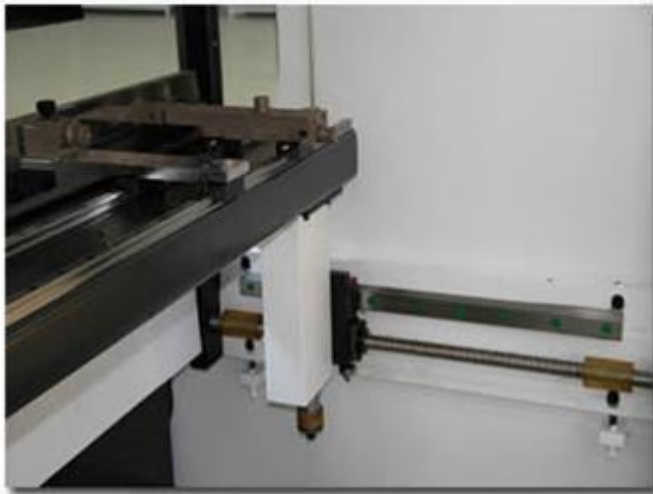
High Accuracy (+/-0.05mm) Ball Screws & Linear Guide Backage
