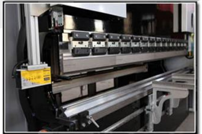
CE Confirm Safety with Laser Beam System
